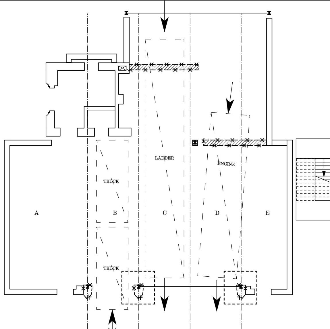
2 C      Ladder and Engine through, moved South wall, column eliminated
