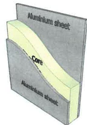
Structure of an ACM sandwich panel. In the case of Reynobond PE, the aluminium sheets' thickness is 0.5 mm (0.020 in) and overall panel thickness is either 3, 4, or 6 mm. [168][169]
